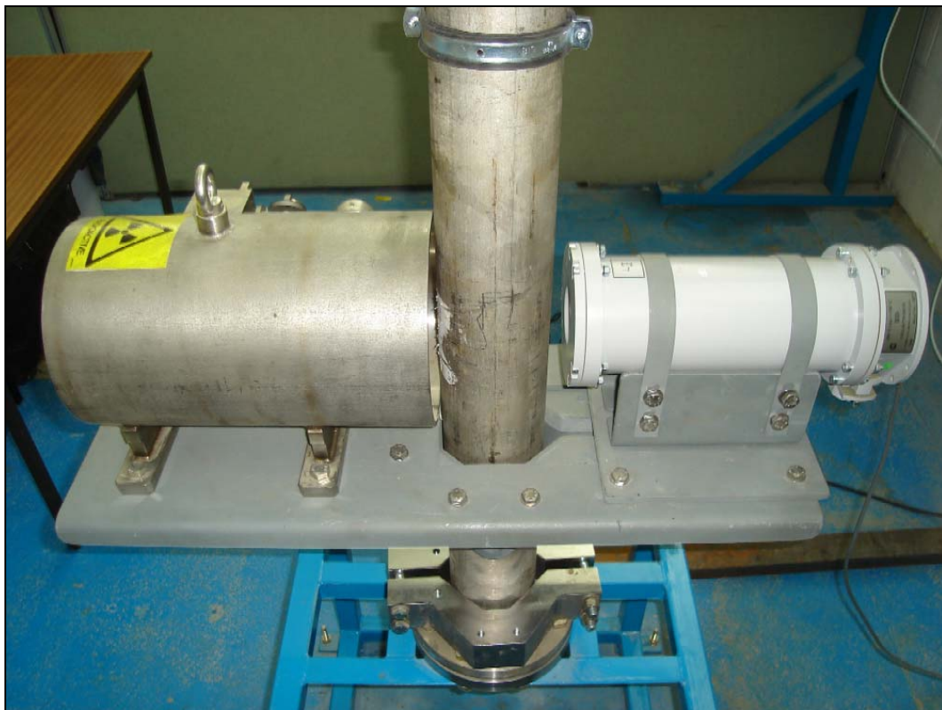
Figure 2 Neftemer comprising Gamma ray source in housing (left) and detector (right)
